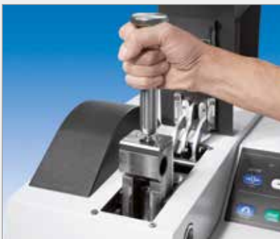
Easy removal of the crusher arm without tools
