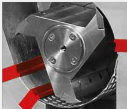
3 double acting cutting bars provide optimum cutting effects (SM 200 & SM 300)
