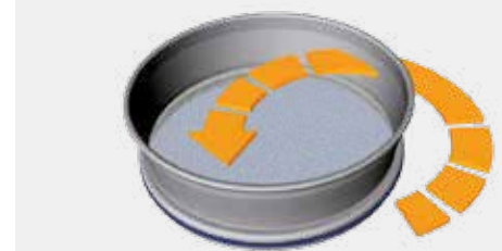
Principle of horizontal sieving
